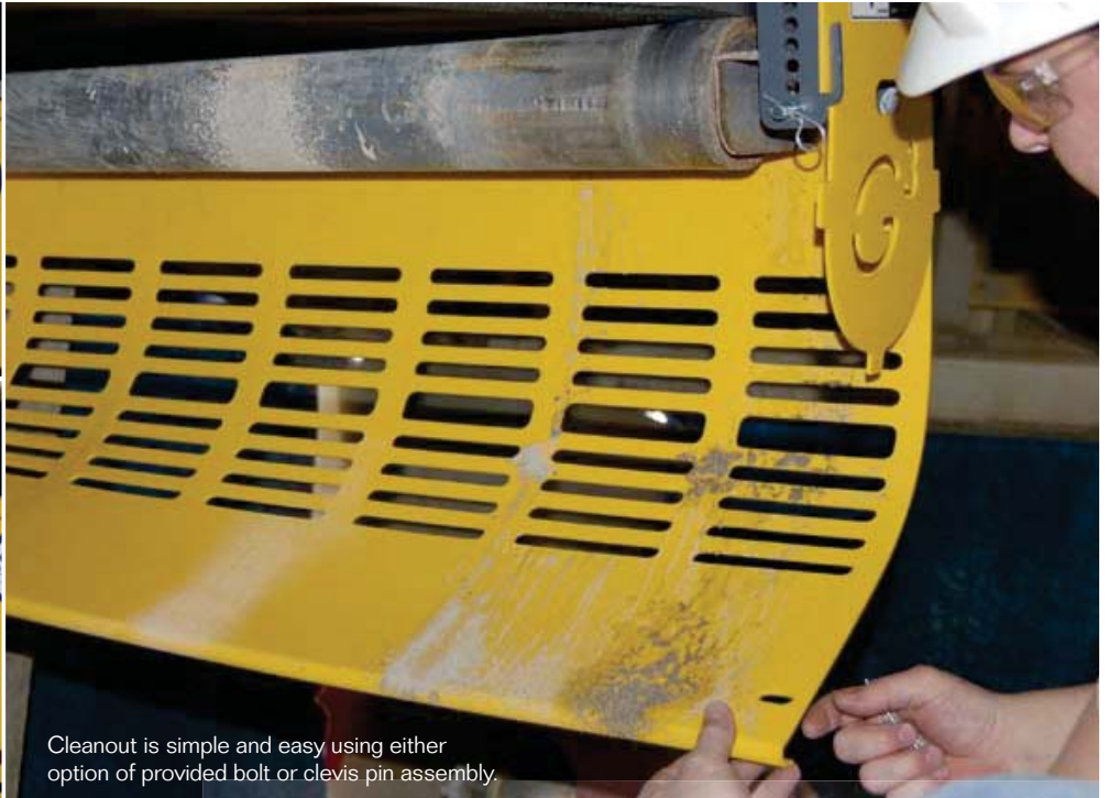
Bolt assembly securely attaches guard on the front side (pinch point) of the roller and may be used on the back side of the roll.
